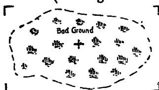
FIG. 4.—To indicate a bad patch in the CENTRE OF AN AERODROME.
