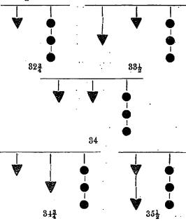
In order to indicate depths of 36, 361, 371 feets etc., up to  $61\frac{3}{4}$  feet, the signals for  $9\frac{3}{4}$ ,  $10\frac{1}{2}$ , 11 feet etc., up to 35½ feet, are respectively shown.
