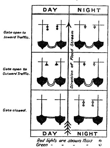
The above-mentioned gate Trawlers will display signals, as shown on the accompanying diagram, to indicate whether the gate is open to inward or outward bound traffic or whether the gate is closed.
